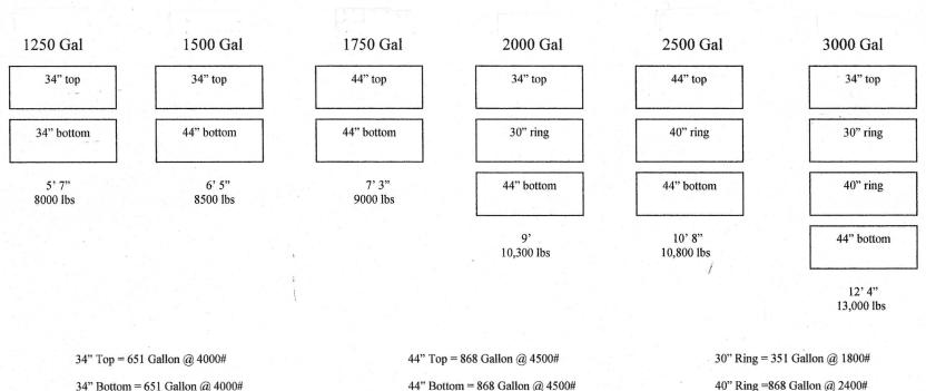
Tanks measurements do not include the cast in riser. Prices do not include delivery charges. The diameter of the water tank is90" Please make your hole a minimum of 9' in diameter
