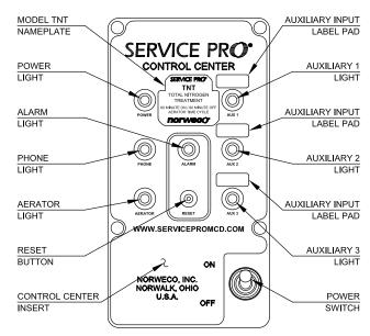
telemetry system shall report the specific condition to the Service Pro monitoring center. In the event that any of the auxiliary inputs detect abnormal operation of the treatment system auxiliary equipment, the audible and visual alarms shall immediately activate and the telemetry system shall report the alarm condition to the monitoring center. The service provider shall automatically be notified by the Service Pro monitoring center of the specific alarm condition using phone, fax or email.
